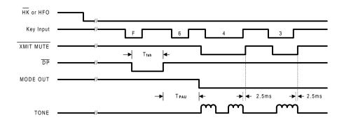
Tfsh: flash time 96 or 640 ms (F1 or F2 respectively) for NT91215 flash time 297 or 640 ms (F1 or F2 respectively) for NT91214
