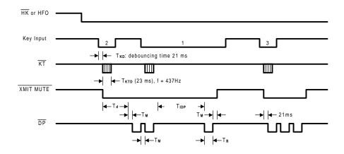
Td: Delay time of Key valid to dialing signal out, typically 0ms
